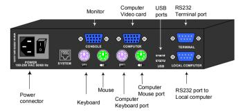
Figure 5 DX User rear panel ports
